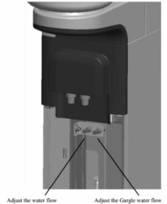
Adjust the Water Flow of Spittoon (If Needed)
